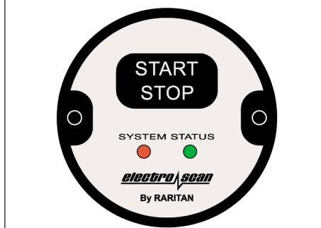
FIG 2 System Status Panel
