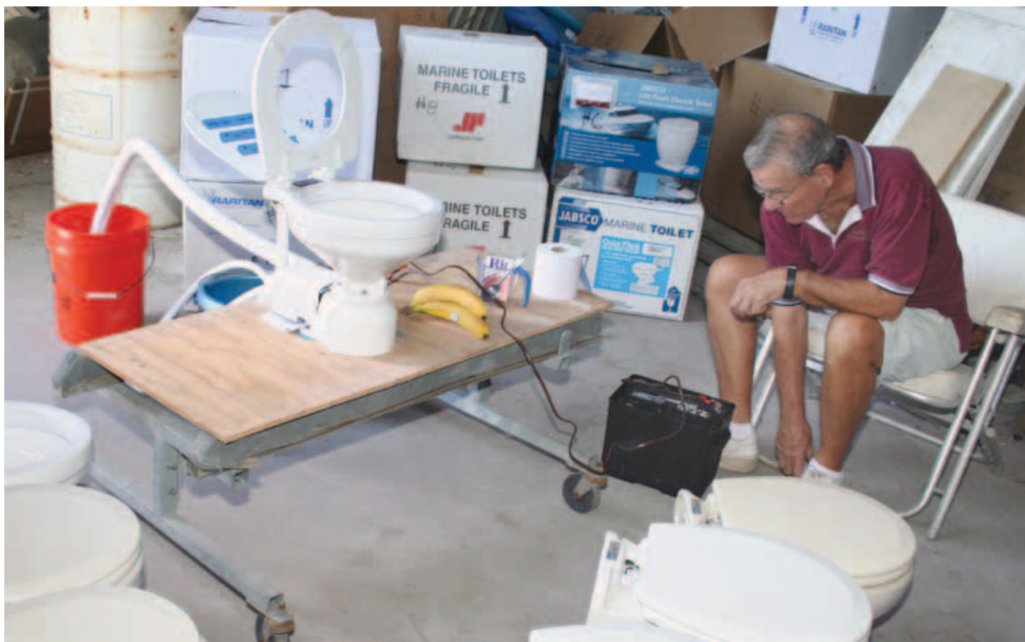
During testing, each toilet's outlet was looped above its bowl, as in an actual installation. The toilets in the first round of testing are sized to replace the compact bowls commonly used for manual-flush marine toilets.
