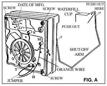
off. If these conditions exists, the module drive mechanism is stuck in the EJECTION CYCLE and the module board #I34M-1 may need to be replaced. If orange wire is not "hot", problem may be with wire harness or other electrical connection(s).
