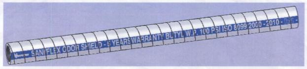
Highest quality marine sanitation hose. Uses Butyl rubber construction which has the lowest odor permeation level not found in other rubber or PVC material hoses. Extremely flexible for easy installation with a low bend radius up to one time its diameter.
