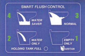
The Raritan Smart Flush Control is a fully programmable flush control. The control allows users to flush the toilet with no water, a small amount of water or a fully timed flush. The timed flush feature can be adjusted on the panel without having to remove any components.
