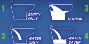
The Raritan Smart Flush Control is a fully programmable flush control. The control allows users to flush the toilet with no water, a small amount of water or a fully timed flush. The timed flush feature can be adjusted on the panel without having to remove any components.
