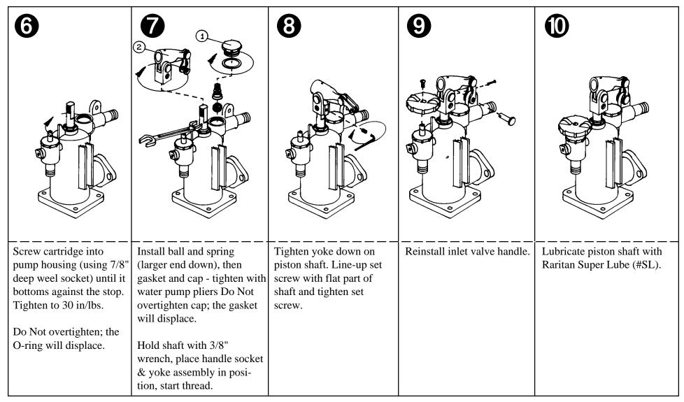
Disassembly - Reverse this process (Steps 6-10). After cartridge is removed, pull piston rod up to raise the seal from its position. Remove piston through the bottom of the pump if necessary.
