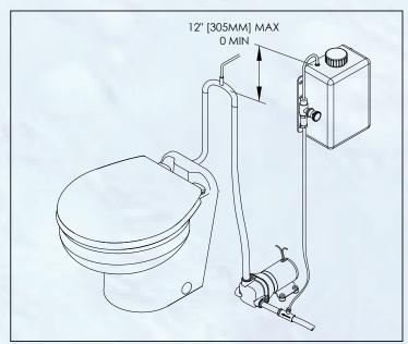
The dispenser tank adds a preset amount of diluted C.P. with every flush. Bacteria introduces by C.P. breakdown organic matters in the inlet hose and bowl rim. This prevents sulfide generating bacteria (rotten egg smell) from growing. C.P. bioactive formula stops the generation of odor without the use of chemicals such as chlorine or formaldehydes.
