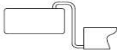
FIG 7 Toilet installed below waterline or below Treatment Device and or holding Tank = Upward discharge flow, Do not remove vent cap
