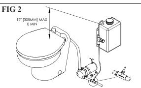
**Electric Toilet above water line - Tank MUST** NOT be mounted higher than 12" above bowl
