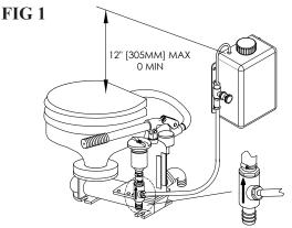
Manual toilet above water line - Tank MUST NOT be mounted higher than 12" above bowl
