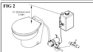
Electric Toilet above water line - Tank MUST NOT be mounted higher than 12" above bowl
