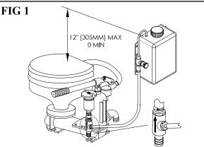
Manual toilet above water line - Tank MUST NOT be mounted higher than 12" above bowl
