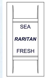
**Sea/Fresh selector -** When both solenoid and remote pump are installed, user can easily select between raw or fresh water
