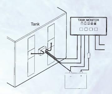
For use on non-conductive tanks (polyethylene, fiberglass, etc.). NOT FOR USE ON FUEL TANKS.
